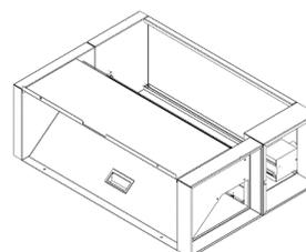
**Energy Recovery Ventilator (ERV):** The energy recovery ventilator harvests energy contained in the exhaust air mixing it with fresh air across a stationary cubic heat exchanger. The filter medium is designed to be pulled out easily for cleaning and replacement.
