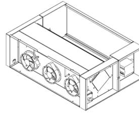
**Economizer:** The economizer uses outdoor air to provide cooling when the outdoor temperature is both cool and dry. It will greatly save energy from stopping the compressor operation.
